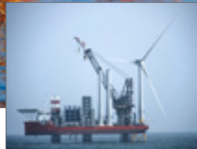
SeaJacks Wind Turbine Installation Vessel Supporting a growing offshore wind industry
